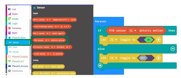
Result: The LED lights on while the motion being detected by the PIR sensor or the LED lights off.
