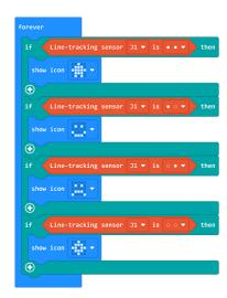
**Result:** Different icons display on the Micro:bit in accordance with the different status detected by the tracking module.
