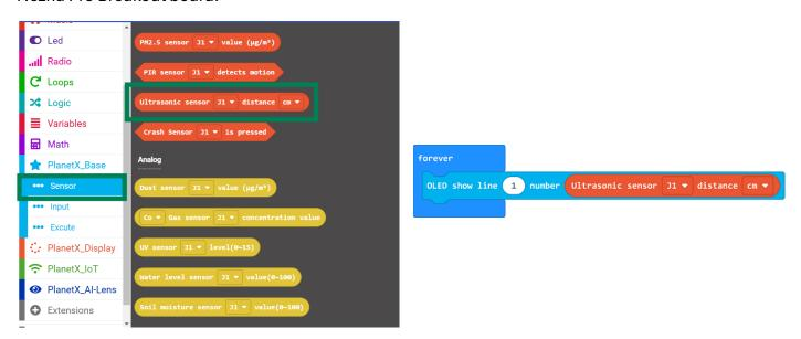
**Result:** The distance value displays on the OLED module.
