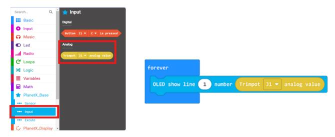
**Result:** The detected value displays on the OLED screen.
