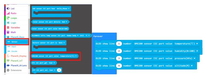
**Result:** The values of the temperature, humidity, air pressure and the altitude in the current environment display on the OLED screen.
