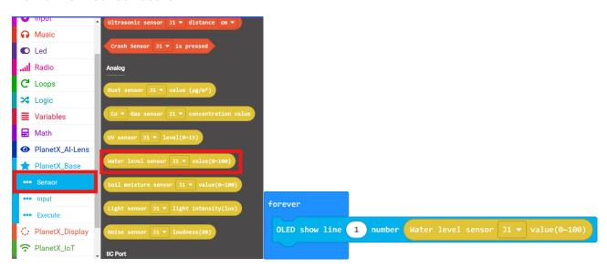
**Result:** The current value of the water level displays on the OLED screen.
