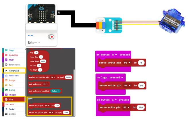
Result: The Servo Motor change it's direction on buttons press and stops by touching Micro:bit logo.
