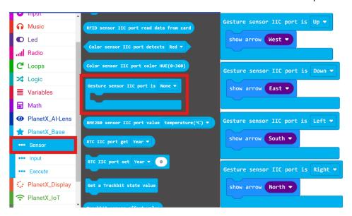
Result: The equivalent icon for each gesture displays on the Micro:bit.
