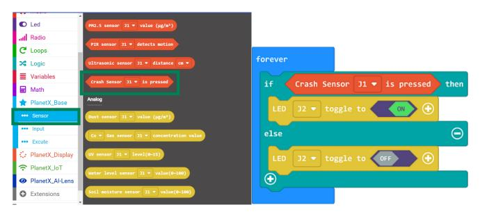
Result: The LED lights on if the crash switch was pressed or it lights off.
