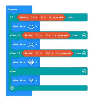
**Result:** The icons display on the Micro:bit accordingly with the order given by pressing button A or B or A+B.
