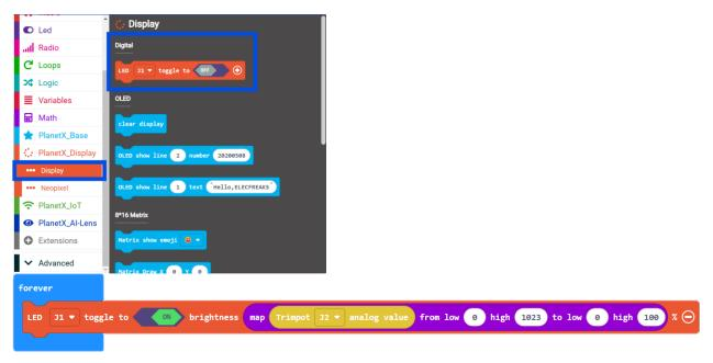
**Result:** The brightness is adjusted by the potentiometer by using a map block which can match Analog Data from 0 to 1023 with brightness from 0 to 100%.
