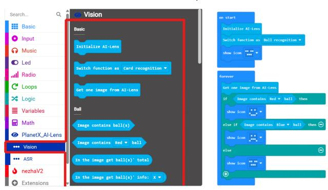
**Result:** A smile face displays on the Micro:bit if the blue ball is recognized by the AI lens and a sad face display on the Micro:bit if it recognizes a red ball. A poker face will be displayed when none of the balls detected.
