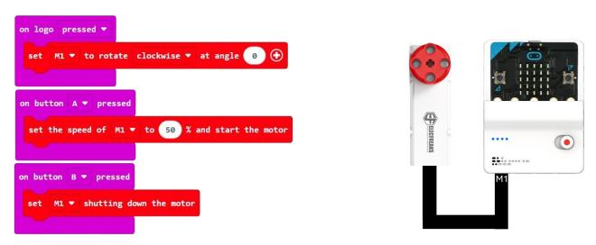
**Result:** When button A is pressed, the motor connected to port M1 starts to move with 50% of speed. When button B is pressed, the motor stops. When Micro:bit logo is pressed, the motor will start to move in its first position automatically.
