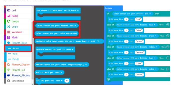
Result: The colour of the detected object displays on the OLED module.
